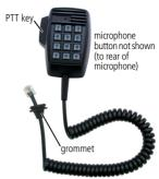
The microphone button operates a hookswitch, which is closed when the microphone is connected to the microphone clip and open when the microphone is removed from the microphone clip. The function of the hookswitch is determined by the radio programming.
